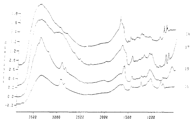
Figure 8. FT-IR spectra of siloxanes 16–19 (hexylamine, benzylamine, methylamine, and dicyclohexylamine analogs of siloxane 1 after treatment with HBr).
